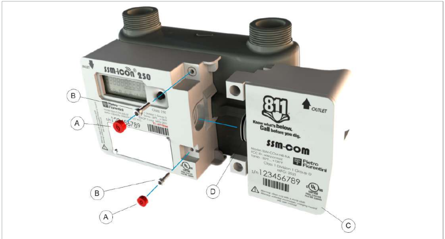
Fig. 9.8. Replacement of the SSM-COM communication module
