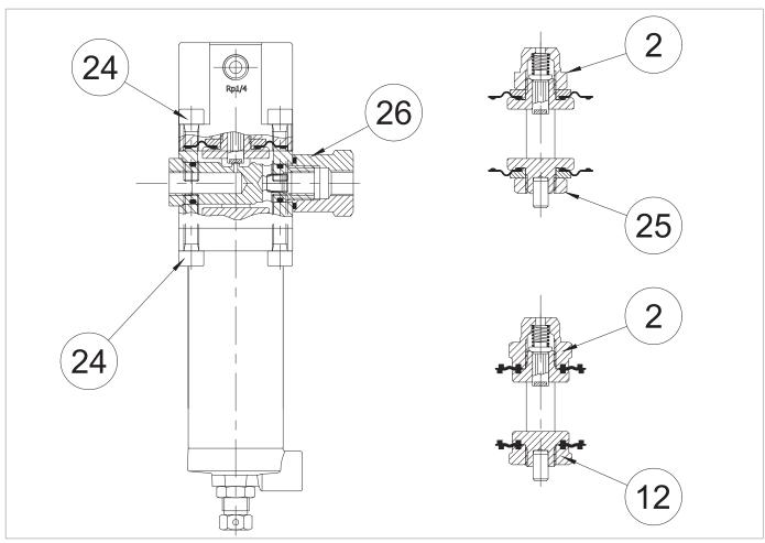
Fig. 9.50. Tightening torques for 204/A pilot
