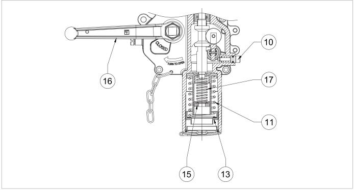
Fig. 8.45. Calibration of pressure switches mod. SA
