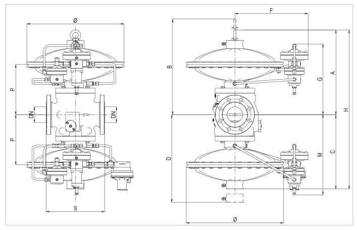
Fig. 5.17. REVAL 182 + PM/182 physical characteristics
