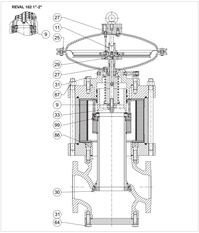
Tightening torques REVAL 182 + Silencer DB/182
