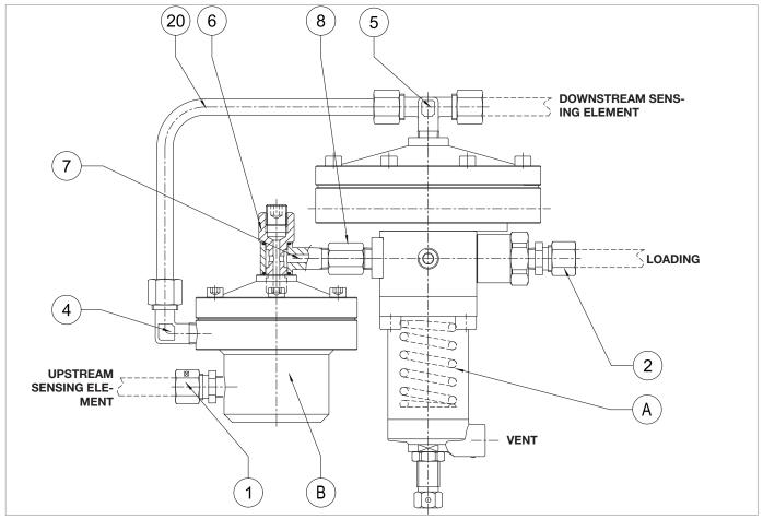
Fig. 9.83. Pilot 201/A and pre-regulator R31/A
