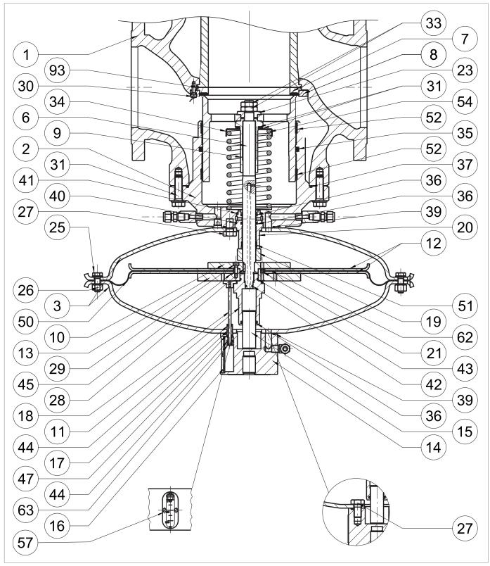
Fig. 9.76. Built-in monitor PM/182 6" ÷ 8"
