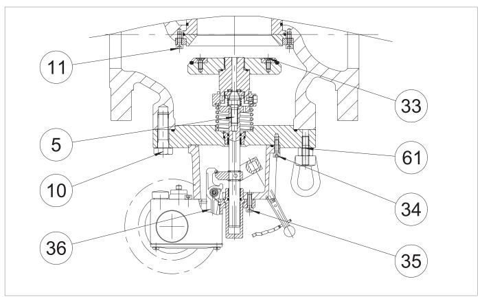
Fig. 9.59. Tightening torques slam-shut valve SB/82 DN 6"-8"
