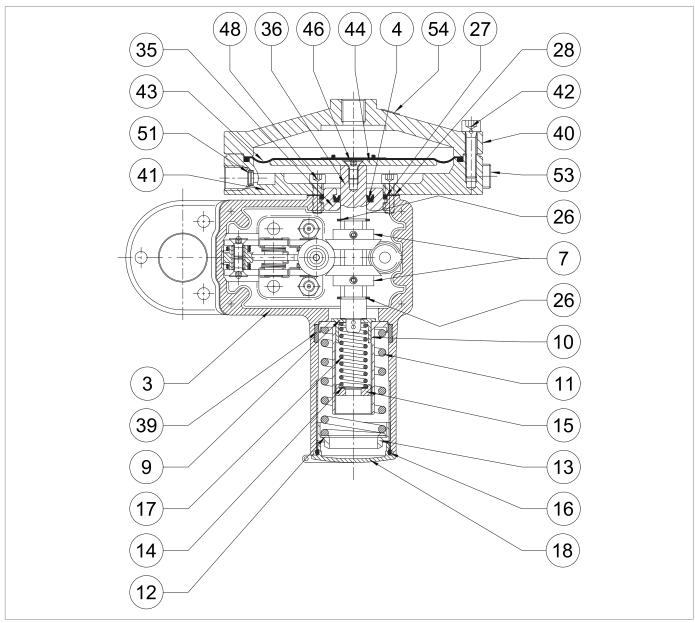
Fig. 9.96. Pressure switch Mod. 101M/101MH
