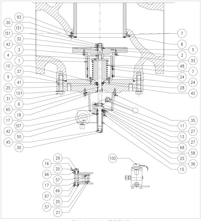
Built-in slam-shut valve SB/82 DN 10"
