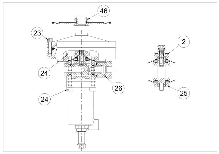
Fig. 9.49. Tightening torques for 201/A pilot
