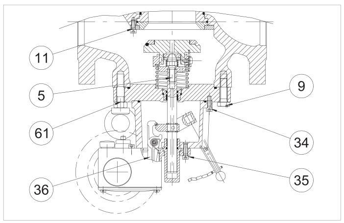
Fig. 9.57. Tightening torques slam-shut valve SB/82 DN 2"  $\frac{1}{2}$  to 4"
