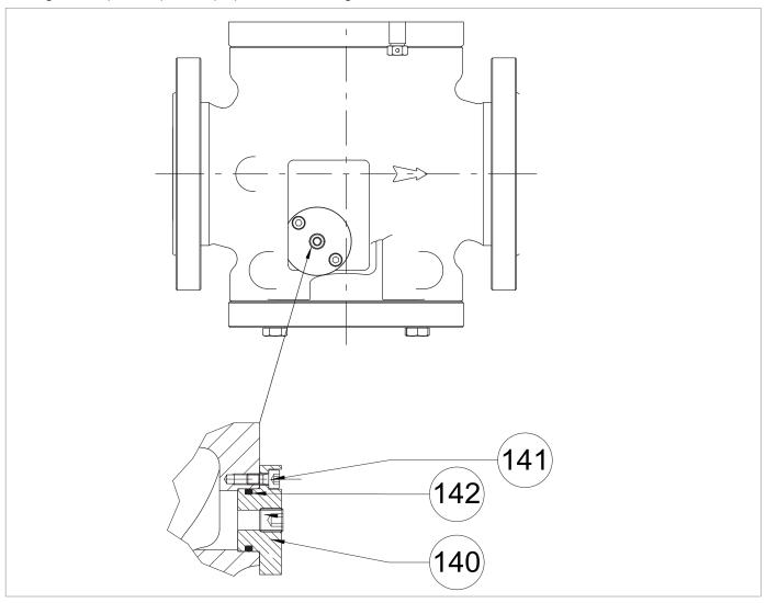
Fig. 9.70. Detail of the regulator cap
