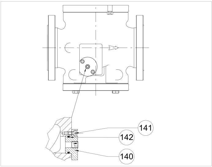
Fig. 9.68. Detail of the regulator cap
