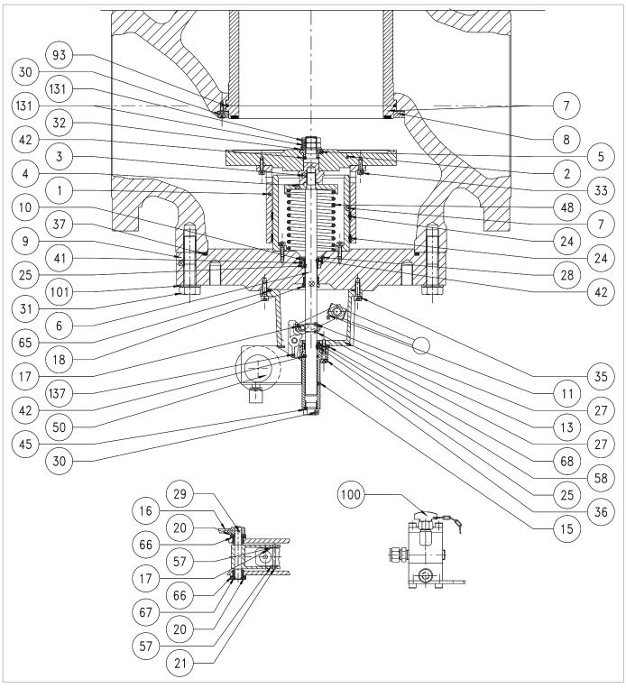
Built-in slam-shut valve SB/82 DN 10"
