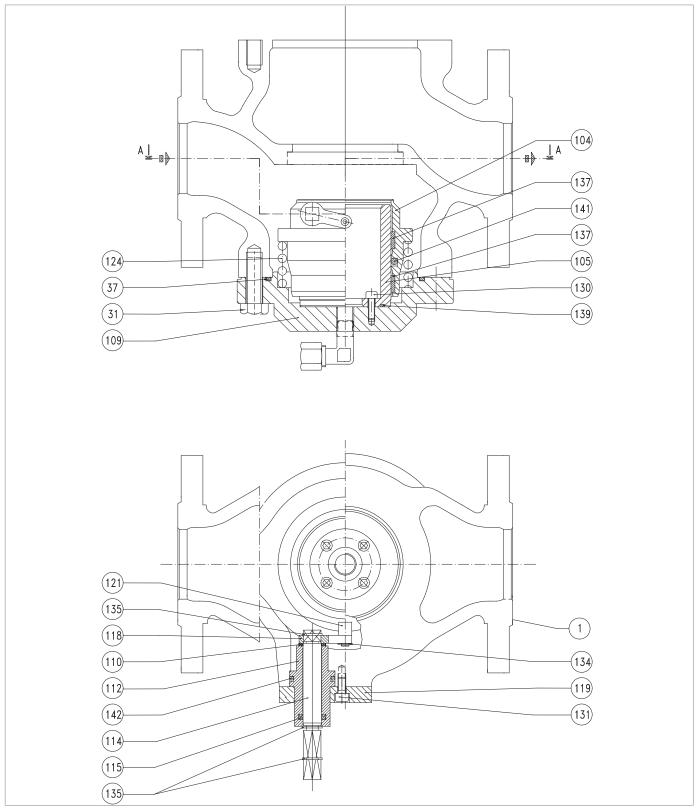
Fig. 9.87. Slam-shut valve SA
