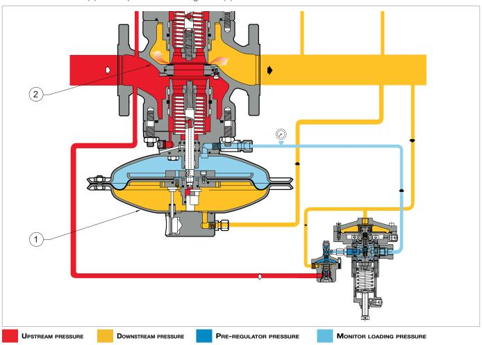
Fig. 4.5. REVAL 182 with built-in monitor PM/182
