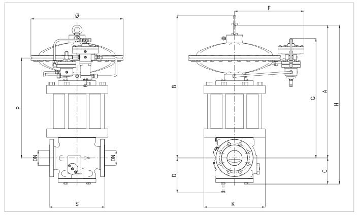
Fig. 5.16. REVAL 182 + DB/182 physical characteristics
