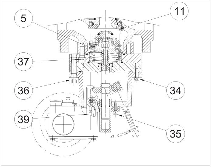
Fig. 9.55. Tightening torques slam-shut valve SB/82 DN 1"
