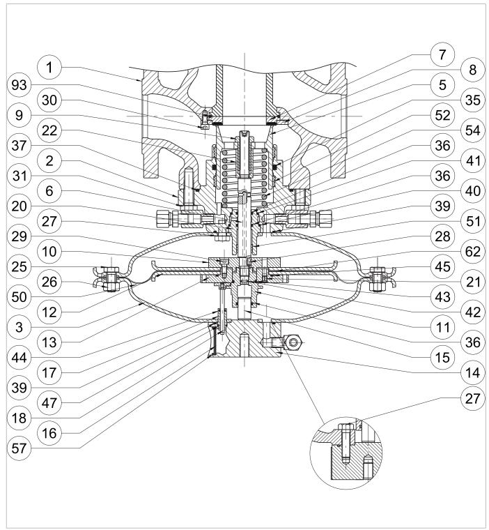
Fig. 9.74. Built-in monitor PM/182 DN 1"- 2"
