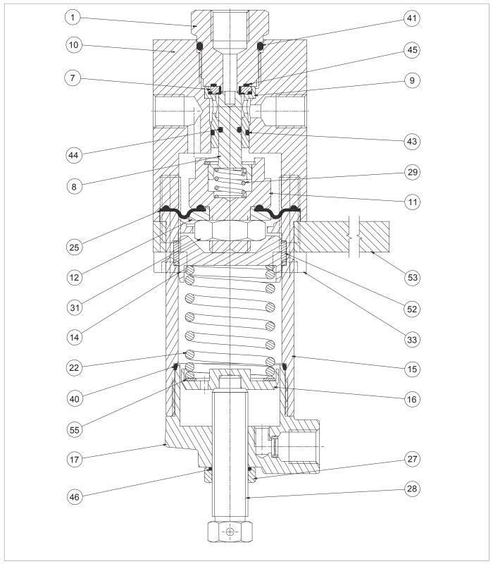
Fig. 9.86. M/A accelerating valve
