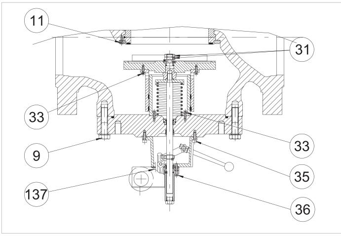
Fig. 9.60. Tightening torques slam-shut valve SB/82 DN 10"
