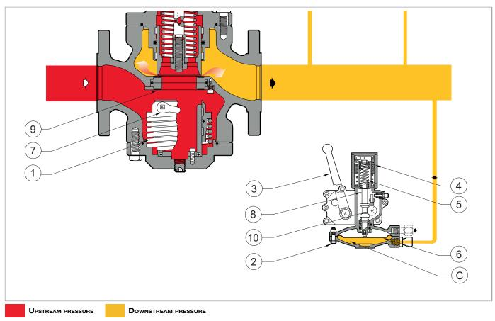
Built-in slam-shut valve SA Fig. 4.11.
