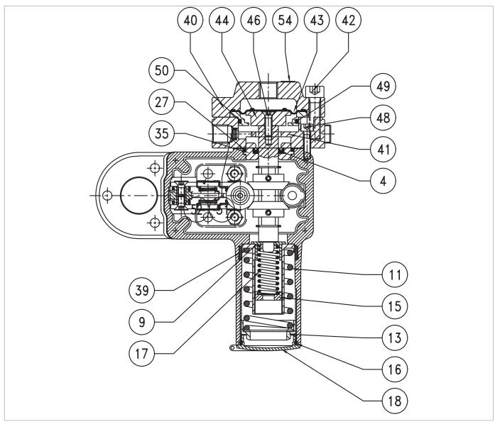
Fig. 9.98. Pressure switch Mod. 103M/103MH
