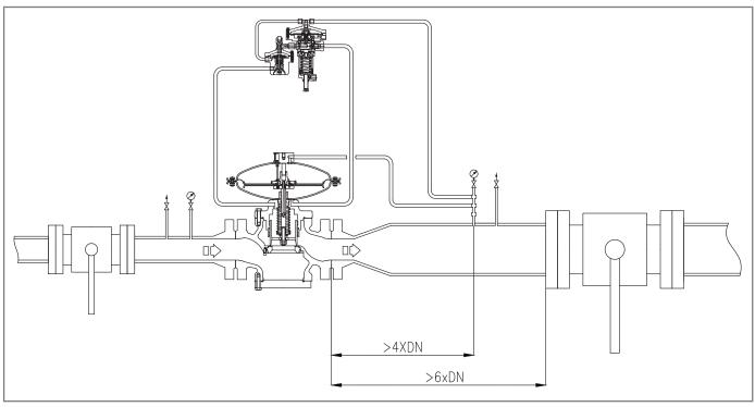
Fig. 6.29. Connection of sensing lines to the downstream piping
