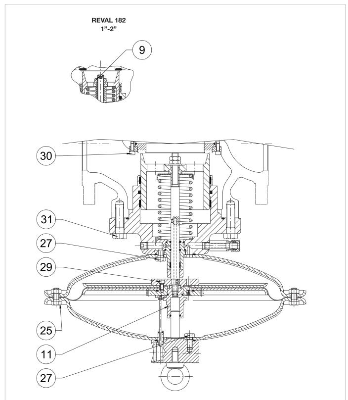
Fig. 9.48. Tightening torques for PM/182 built-in monitor
