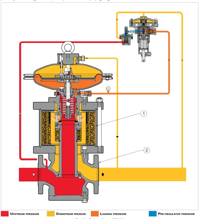
Fig. 4.3. Built-in silencer DB/182
