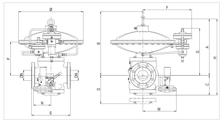
Fig. 5.18. Physical characteristics REVAL 182 + SA
