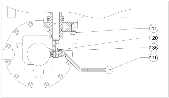
Fig. 9.91. Pressure switch mod. SA
