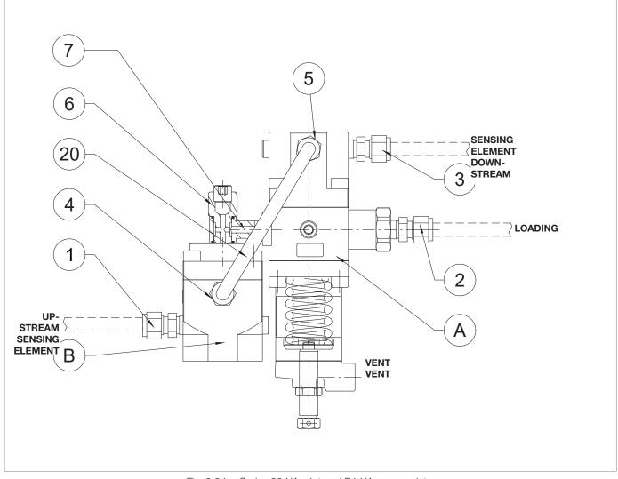
Fig. 9.84. Series 204/A pilot and R14/A pre-regulator
