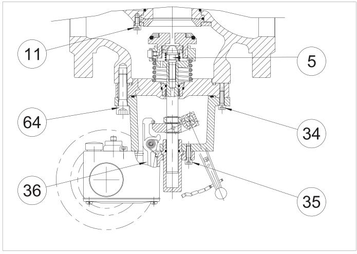
Fig. 9.56. Tightening torques slam-shut valve SB/82 DN 2"
