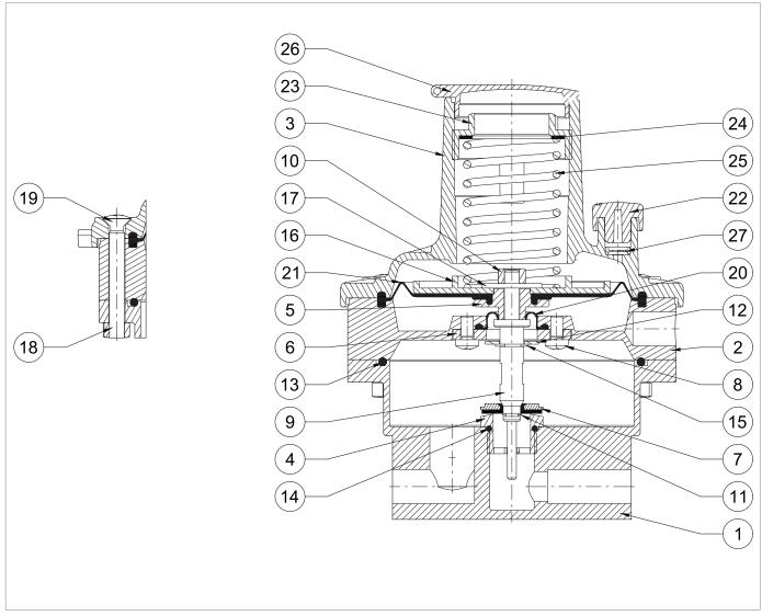
Fig. 9.85. V/25 accelerating valve
