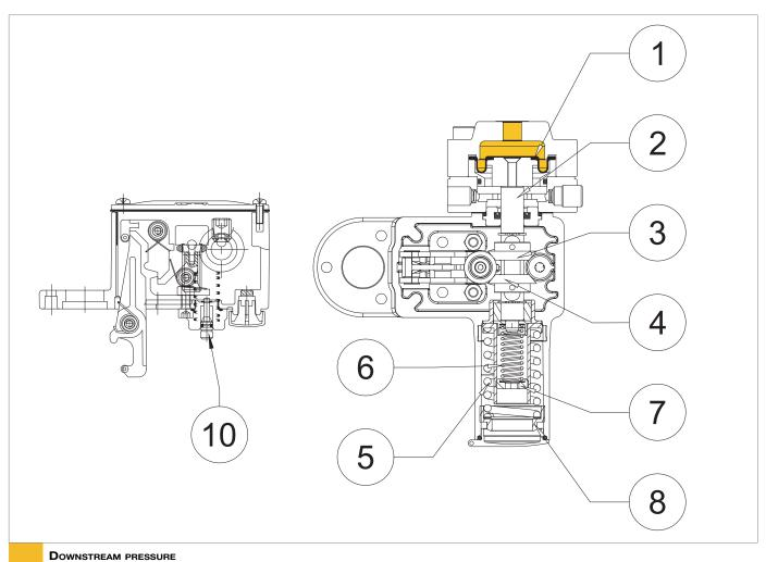
Fig. 4.14. Slam-shut device pressure switch
