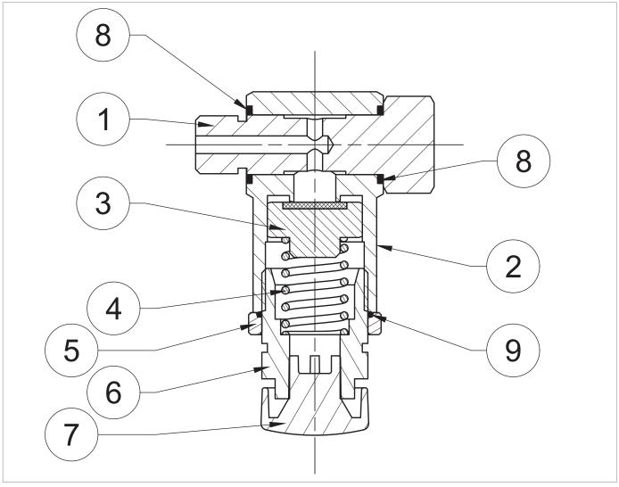
Fig. 9.104. Safety valve VS/FI for LINE OFF 2.0
