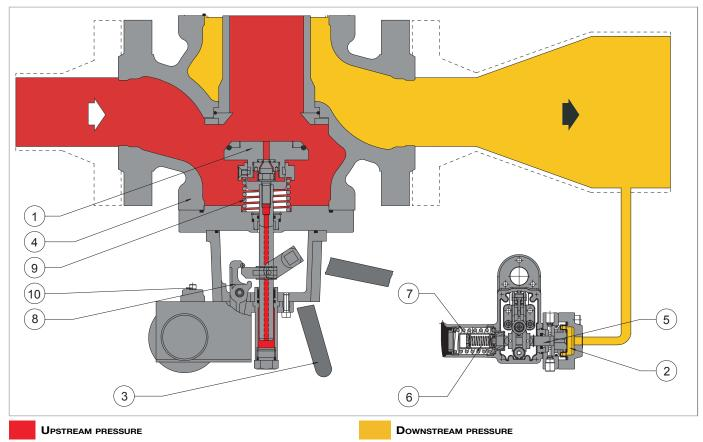
Fig. 4.12. REVAL 182 with SB/82 incorporated slam-shut valve
