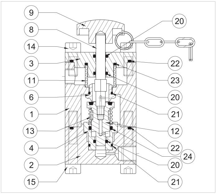
Fig. 9.101. HP2/2 bypass device
