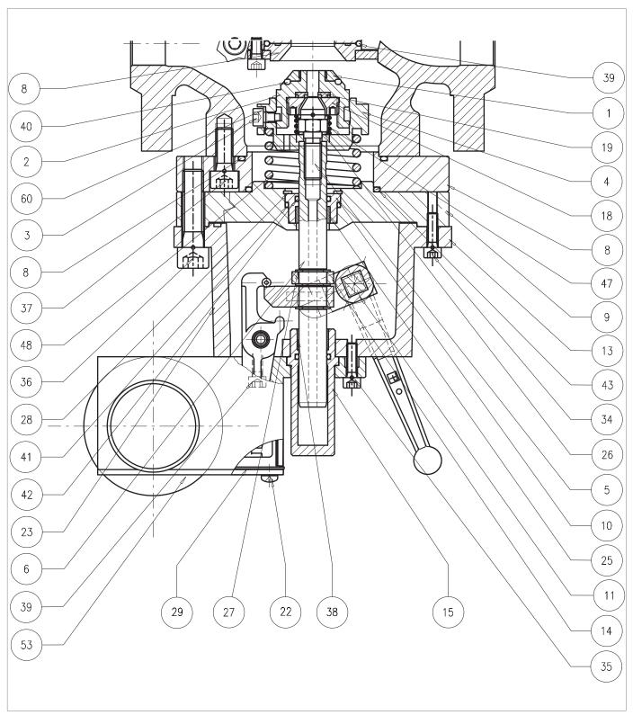
Fig. 9.92. Built-in slam-shut valve SB/82 DN 1"
