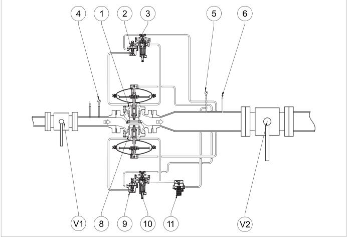
Fig. 8.34. Commissioning of the REVAL 182 regulator with built-in monitor PM/182 and V/25 accelerating valve
