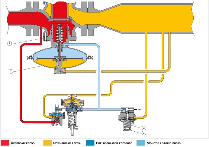
Fig. 4.9. V/25 accelerating valve
