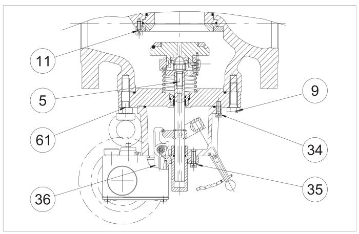
Fig. 9.58. Tightening torques slam-shut valve SB/82 DN 2"  $\frac{1}{2}$  to 4"
