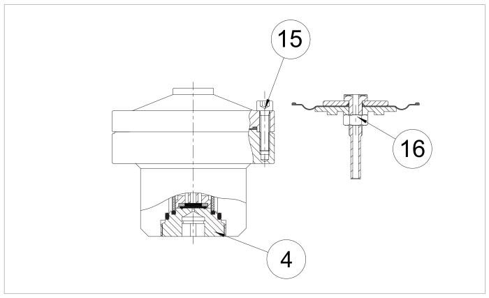
Fig. 9.51. Pre-regulator R31/A tightening torques
