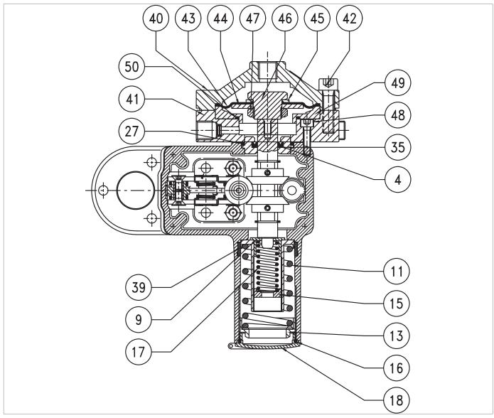
Fig. 9.97. Pressure switch Mod. 102M/102MH
