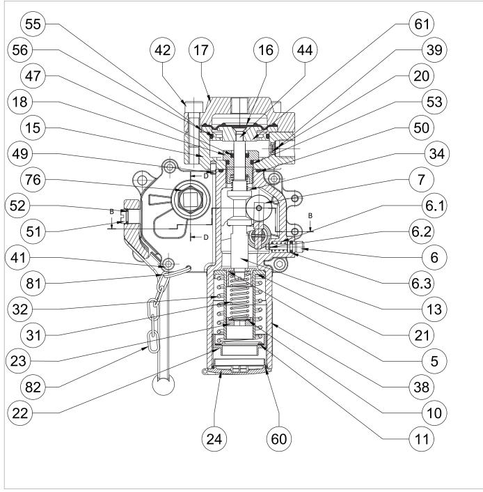
Fig. 9.90. Pressure switch SA-93
