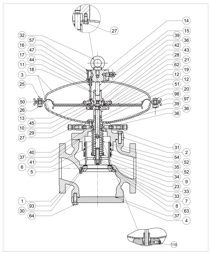
Fig. 9.69. Regulator REVAL 182 DN 2" 1/2 to 4"
