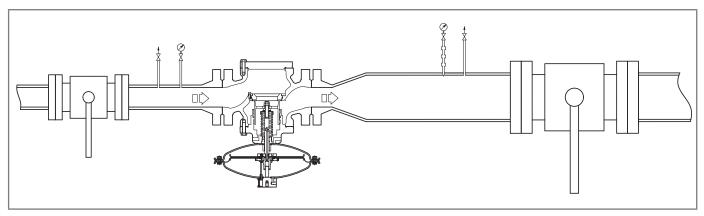
Fig. 6.28. Inverted position
