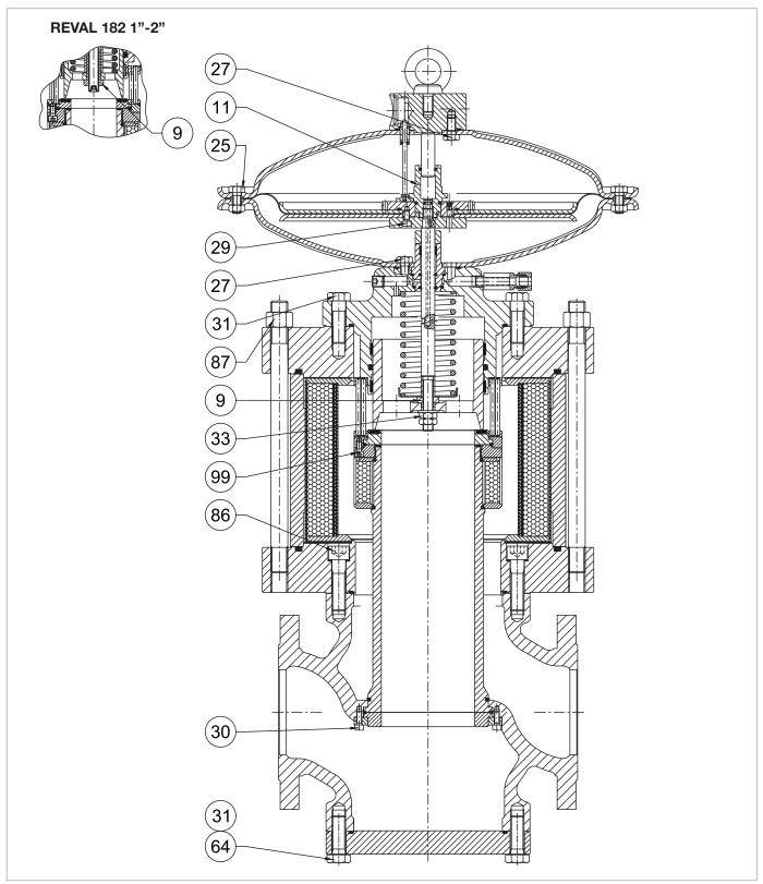
Fig. 9.47. Tightening torques REVAL 182 + Silencer DB/182
