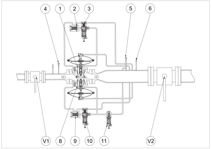
Commissioning of the REVAL 182 regulator with built-in PM/182 monitor and M/A accelerating valve Fig. 8.35.
