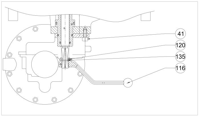
Fig. 9.88. Pressure switch mod. SA
