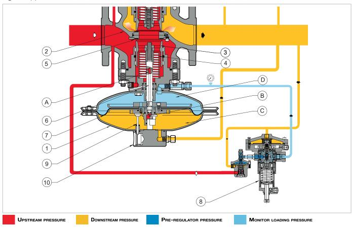
Fig. 4.6. Built-in monitor operation
