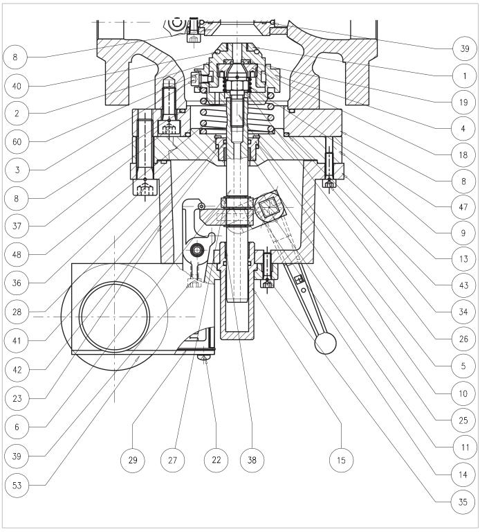
Built-in slam-shut valve SB/82 DN 1"
