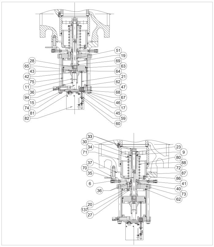
Fig. 9.100. HB/97 built-in slam-shut valve
