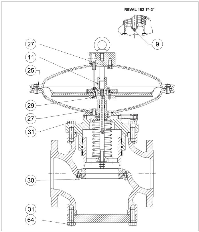
Fig. 9.46. Tightening torques REVAL 182
