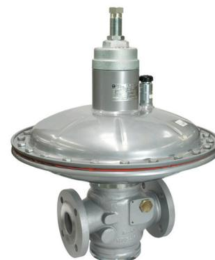
The **Norval** by Pietro Fiorentini is a **direct-operated** gas pressure regulator. Suitable for use with previously filtered gaseous fluids, it is mainly used for medium and low pressure natural gas distribution networks. It is classified as **Fail Open** according to the European Standard EN 334. The Norval is **Hydrogen Ready** for NG-H2 blending.
