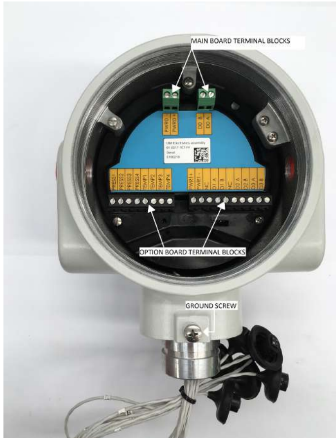
Figure 3-3 - FSN Series electrical interfaces shown with RS485 and PT option board
