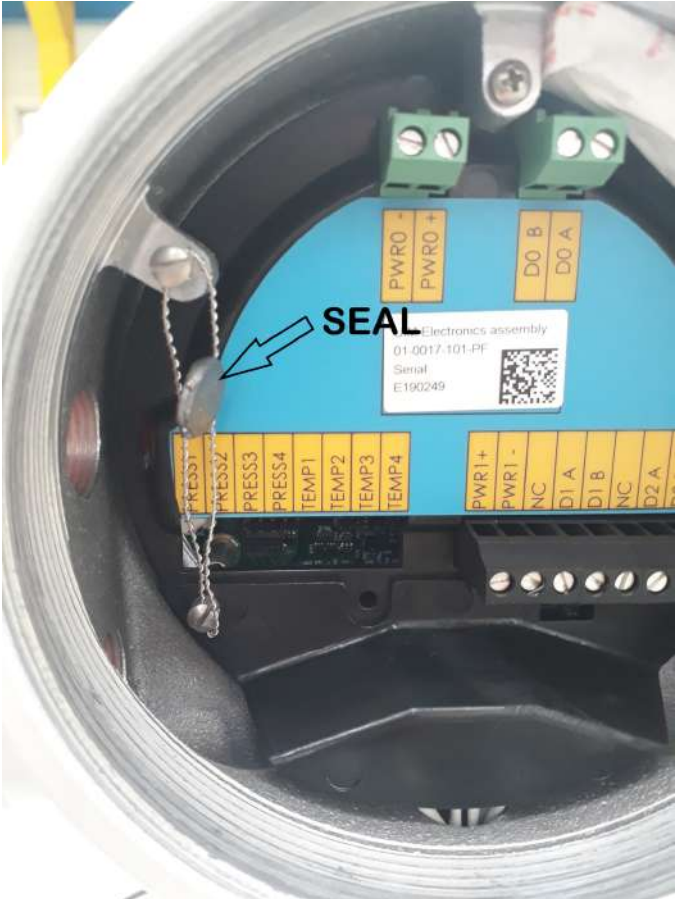
Figure 2-2: Electronic assembly and transducer connector cover seal
