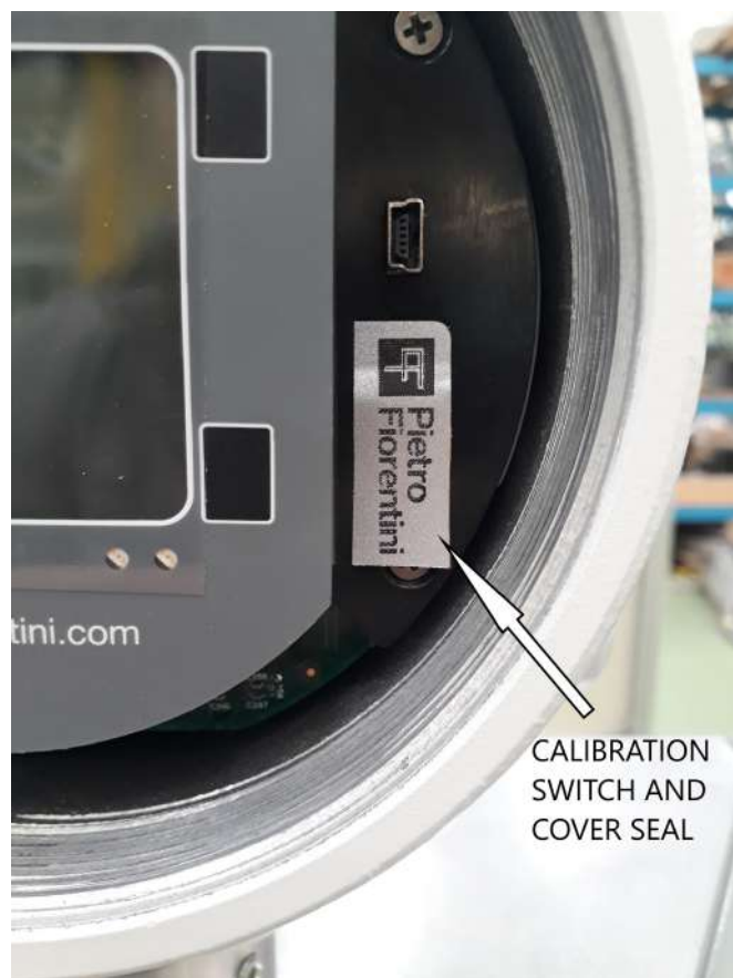
Figure 2-4: Calibration Lock Switch and Display Cover Seal
