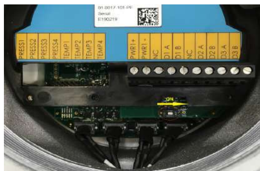
Figure 5-1 - Line termination resistor switch
