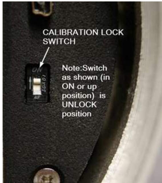
Figure 2-3: Calibration Lock Switch
