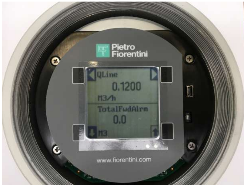
Figure 6-1 - LCD and keypad (front cover removed)
